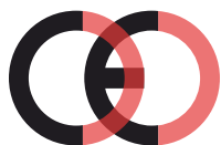
False CE Mark (too close)
