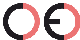
False CE Mark (too far)
